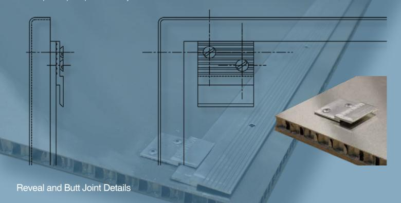
Reveal joints allow for the addition of complementary or contrasting elements between the panels. Wood veneers or colored stainless can be used to create a wide variety of effects. Reveal panels, below left, are 304 stainless steel with non-directional polish.
