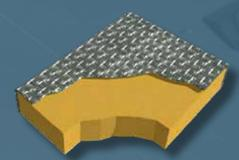
Solid cores include premium fire rated MDFB laminated with a fire-rated adhesive. Plywood and standard medium density fiberboard are also available. Panel thicknesses are from 1/2" to 2".
