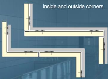
Corners can be detailed by overlapping panels or by fabricating panels "formed" with both inside and outside corners. Formed outside corners can be combined with butt inside corners to save cost and ease installation.
