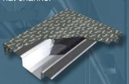
Hat channels are metal elements that stiffen panels and provide mounting points for the attachment of Z-Clips. A feature of hat channels is the ability to create deeper panels (up to 2") without adding significant weight to the assembly.
