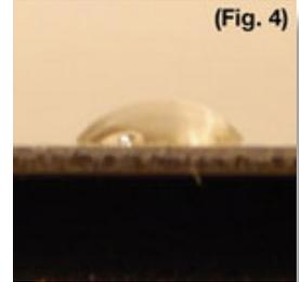
Surface irregularities can help by preventing contact between foreign liquids or solids and the surface. Less contact implies lower contact angle, which implies less adherence. Grosser irregularities such as #4 polish and Linen finish stainless steel provide varying angles to help increase wetting, which is undesirable.
